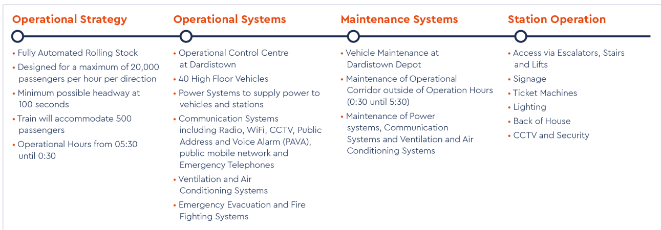
Diagram 18.2 Summary of Key Activities during the Operation Phase of the proposed Project
